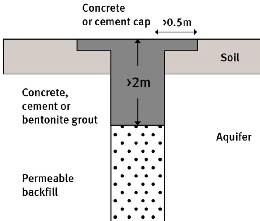
**Figure 2: Schematic diagram for borehole seal and cap**
